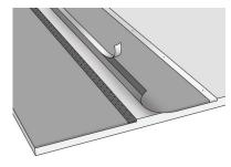
Lay out the underlay membrane in the direction of the verge in a straight line and slightly over the edges so that the edges can be folded approximately 15 mm under the lower edges of the boarding. Nail the top edge at every 100 mm (start the nailing from about 200 mm of the edge that has an adhesive strip on the bottom side).
