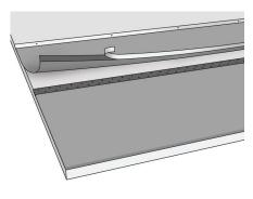
Lay out the membrane in a straight line on the lower eaves and slightly over the edges so that the edges can be folded approximately 15 mm under the lower edges of the boarding. Pre-nail at the top edge at approximately every 1 m through the protective plastic cover of the adhesive strip on the top side. Lift up the lower edge of the membrane, remove the protective plastic cover of the adhesive strip, and press the membrane tightly
